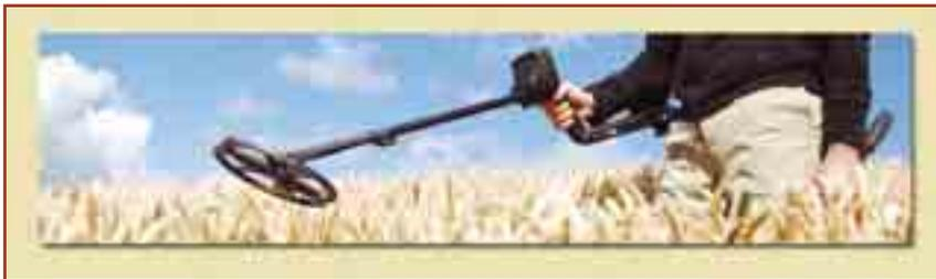
can immediately be established whether or not there is any metal buried beneath a building or under the ground. These detectors, which make it easy to find buried metals such as gold, silver, copper and bronze, are frequently employed in engineering, construction and by the military, and by others for treasure hunting.
